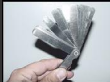
Feeler Gauge - A very useful and very necessary tool for valve adjustments
