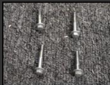
Do yourself a favor and place the side cover bolts on the ground in the order you removed them. This keeps you from guessing what length goes where.
